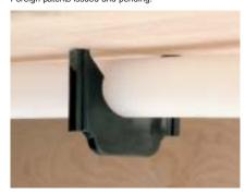
RB Clip housings are manufactured of high-density polyethylene that is lightweight yet strong. Two galvanized nails per clip are driven 5/8" into the wooden surface, providing an installation that is both strong and permanent.
